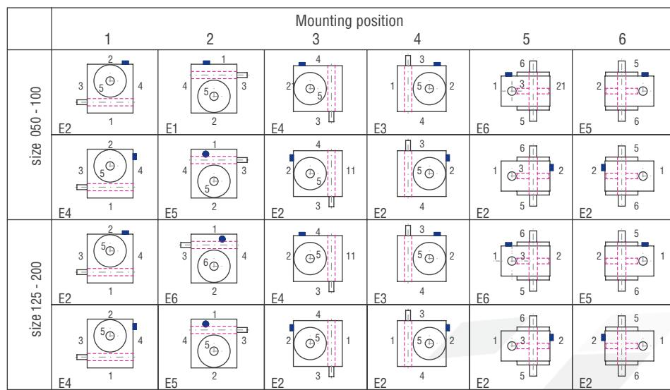
Figure 8.2.9-1; Installation positions
