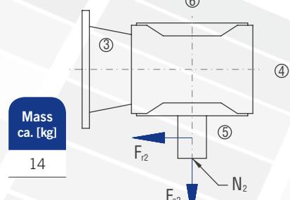
The mass of the gearbox may deviate depending on the flange size, the type and the gear ratio.
